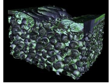
Due to the self developed foamable alloys and the foaming method **our foams** became **castable**, **well machinable**, weldable, fire and water proof.
