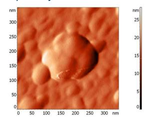
NTEGRA Prima AFM high resolution image from a discrete HIV virus (sample was 3 µl)
